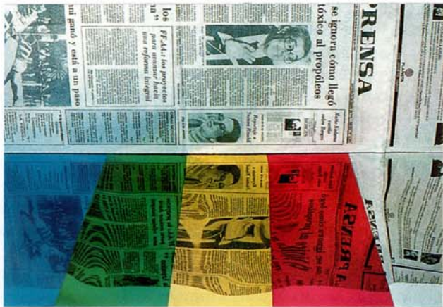
FIG. 6. Specular reflection having spectral selectivity. Five sheets of metallized polyester—four colored (blue, green, yellow, red), and one colorless—are placed so as to reflect the page of a newspaper. Only the colorless mirror has no spectral selectivity; the others absorb certain wavelengths and produce a specular reflection of the remaining ones.
